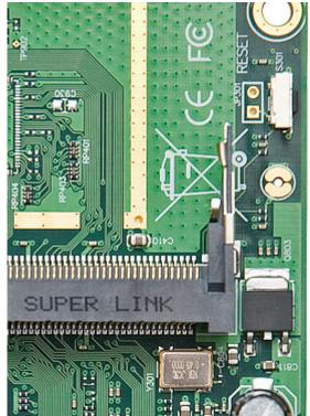
To reset RouterOS config Hold metal object in here while the board boots.
